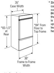
Shipping height. The refrigerator can be adjusted to fit into a cutout that is 83-1/2" min. to 84-1/2" max. height. Note that the top case trim at the front is 1/2" higher and will overlap upper cabinetry or soffit. Use leveling legs and wheels for height adjustment.
